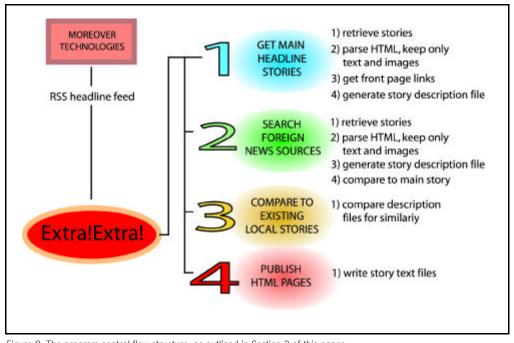
Figure 9: The program control flow structure, as outlined in Section 3 of this paper  $% \left( 1\right) =\left( 1\right) \left( 1\right) \left($
